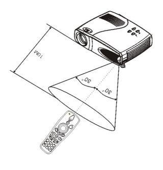
The projector is equipped with an IR Transceiver located at the front cover of the unit for the receipt of remote control transmission.
